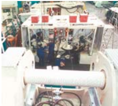
Hydraulic pumps are fitted to a RH 200 module
